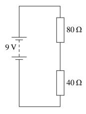
(a) Calculate the potential difference across the 40  $\Omega$  resistor.
