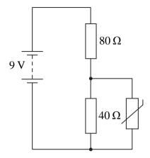
The thermistor is initially at a temperature of 100  $^{\circ}$ C and its resistance is 20  $\Omega$ . As the thermistor cools down, its resistance increases.
